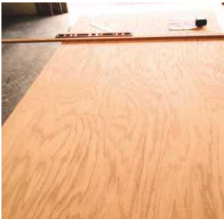
STEP 1. The first step is to cut 20mm plywood for the top and bottom of the TV stand
